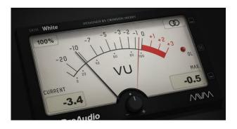
The VU meters indicate the output volume, with either a needle or LED lights. The VU meters are colour coded to differentiate between ideal levels and those that are too high. Occasionally peaking the volume is acceptable, but ideally your volume should stay out of the red. Some VU meters make an audible clicking sound when peaking.
